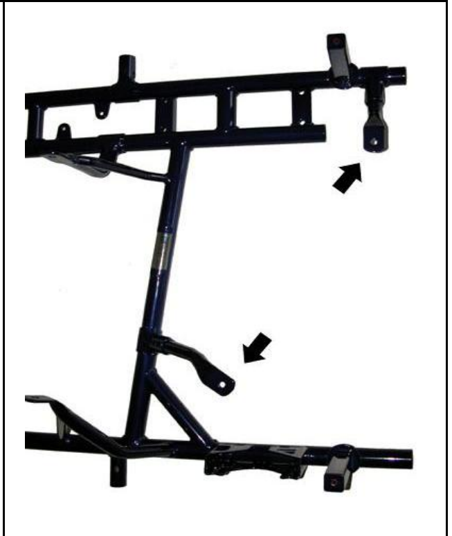
Photo from above of the frame with the section of the two supports for the exhaust system
