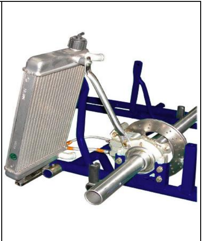
Photo of the frame from the side with the section of the supports for the radiator (radiator mounted)
