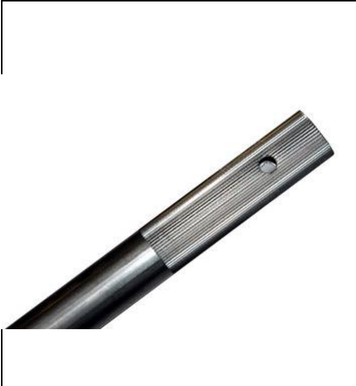
Photo from the steering column with the section with the knurling for the steering wheel hub (knurling according to DIN 82 - RAA1).
