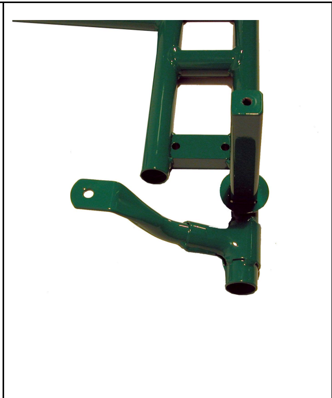
Photo of the frame from the back with the section of the support for the RTPS (Rear Tire Protection System)
